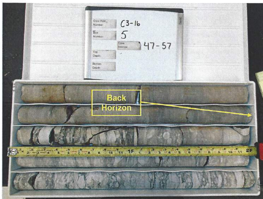
Photograph 3. Tunnel Back Horizon - Core Hole C-3
