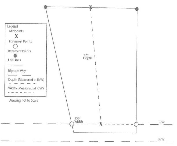
Depth to Width Ratio Calculation
